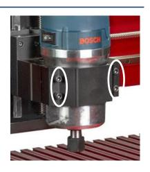
2. Loosely attached the spindle mount with the four new mounting bolts. Tighten the two bolts on the right side. Slide the spindle into the mount so it is positioned about midway, or a height that meets your needs. Tighten the two left-hand bolts.
