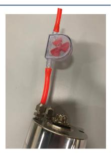
4. Slide one of the hose nuts onto the short section of hose below the flow meter and then onto one of the hose nipples on top of the spindle.
