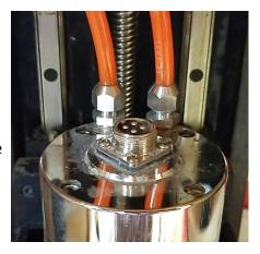
6. First run the pump power cable through the grommet from the bottom side of the lid, then run the hoses through the grommet from the top side of the lid.
