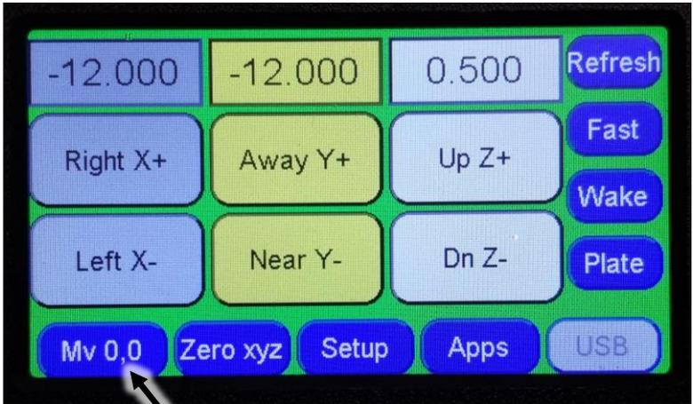
The X and Y positions on the main screen will read the negative offset positions. Next, press **Mv 0,0** to move the XY axes to the new “project” zero location (see below)
