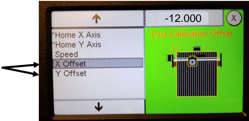
The **X Y Offset** options allow you to set the XY zero location a precise distance from the machine's Home position. This new location can be referred to project zero because it matches the XY datum location in your VCarve Job Setup.
